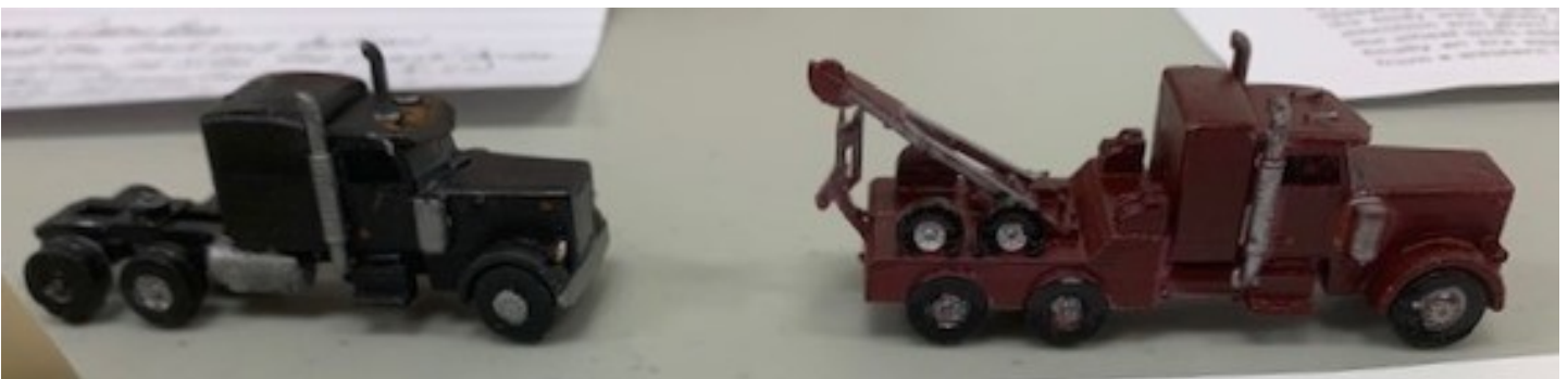
Above: Jimmy Braum won third place for his tractor cab and heavy duty tow truck. He 3-D printed these models from files he found on "Thingiverse"; then primed the cabs, airbrushed them, and then hand-painted smaller details (like lights) with a brush.
