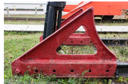
Prototype photo of the wheel chock Ken and Tom used as the basis for their design of the model; photo by Steve Boyko, blogging at "traingeek.ca".
